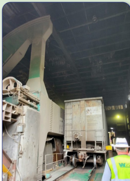
A railcar tipper prepares to rotate 65 tons almost 180° to dump trash onto the tipping floor.
