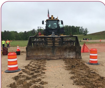
A landfill compactor backs through barrels that are placed slightly wider than the front blade
