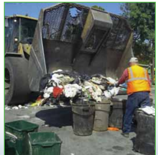
A selected load is transferred into containers for weighing 200 lb. samples at Baltimore City's Northwest Transfer Station
