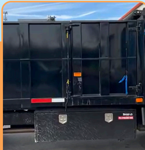
GCI specialty trucks, with compartment near the front of the truck, to provide separate areas to preserve materials from being crushed/contaminated for reuse/recycling
