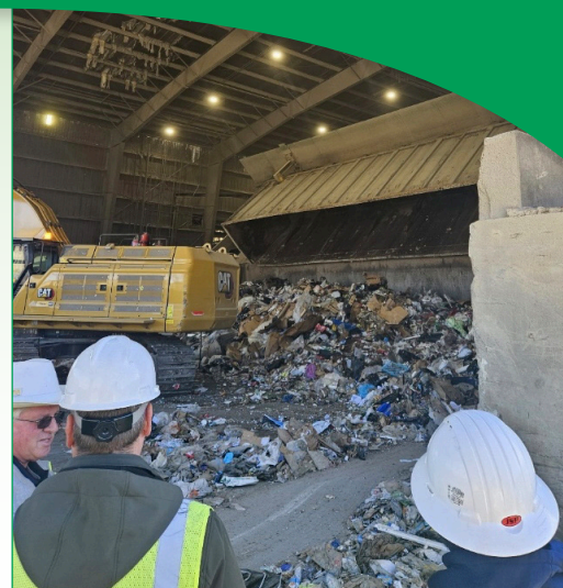
The Authority's James Woods (right) observes as the tipper tilts the rail car and waste falls to the tipping floor.
