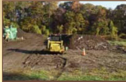
Veterans Composting is a farm based operation in Harford County that uses aerated static piles for composting of the food scrap and wood.
