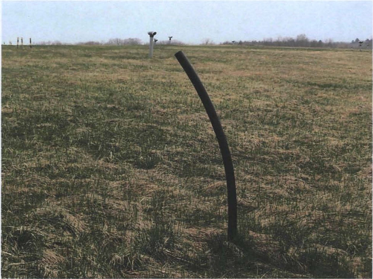
Figure 8. Rubber casing protecting one of the most recent settlement gauges.
