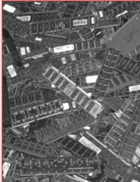
Computer Boards which are recycled to recover precious metals (gold & platinum).
